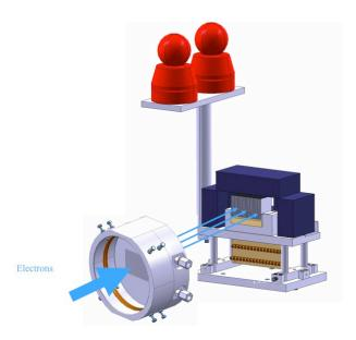
**Fig. 5.240:** Segmented beam dump assembly with a 20 cm long multi-slit collimator (32 vertical slits, each 400 um wide) made out of iron and 32 tungsten segments, 2 mm wide and 5 cm long, spaced by 1 mm. Radiation hard ceramics are used as insulating material between plates.
