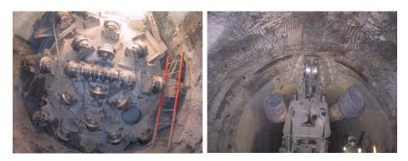
Fig. 6.5: TBM (Gripper) type machine (left). Roadheader type machine (right)
