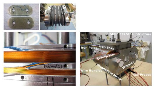
Fig. 5.30: Left: Manufacturing process of short-model wiggler. Right: Measurement configuration of wiggler in mirror configuration.
