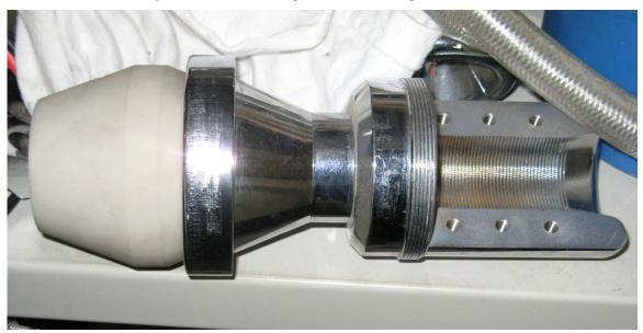
Fig. 5.262: New feedthough connector developed at KEK/ATF
