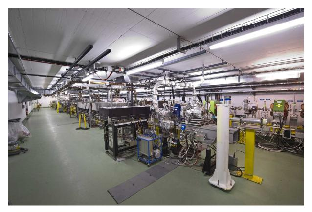
Fig. 7.26: Photo of the CALIFES Probe Beam linac installation in the CLEX hall [27]
