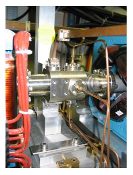
Fig. 5.222: Button pickup 'BPR' installed in the CTF3 Combiner Ring
