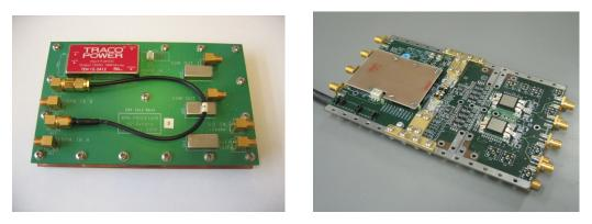
**Fig. 5.332:** Prototype modules for the IP Feedback system: a BPM signal processor (left) and an integrated feedback circuit and drive amplifier (right)
