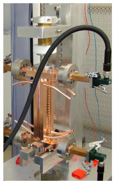
Fig. 5.86: RF measurement set-up of a test accelerating structure
