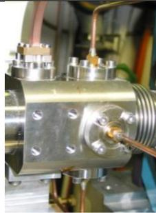
Figure 41: Button Pickup “BPR” installed in the CTF3 combiner ring
