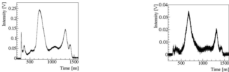
Figure 40: CDR power signals measured with two SBD detectors: DXP-08 40 - 60 GHz (left) and DXP-12 60 - 90 GHz (right) [lix].
